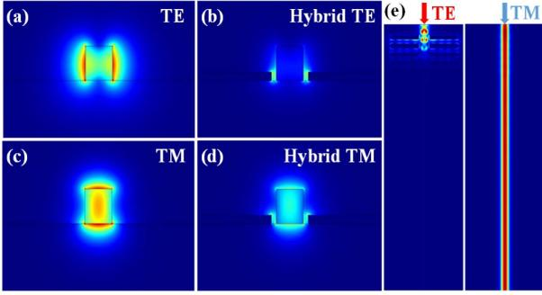
Fig. 4. Normalized electric field distributions of (a, c) dielectric TE and TM mode; (b, d) hybrid plasmonic TE and TM mode. (e) Power distribution along the propagation direction from top view when TE and TM mode is injected respectively. Here,  $W = 280$  nm,  $g = 50$  nm, and  $h_m = 85$  nm.
