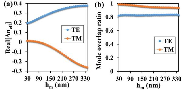
Fig. 3. (a) The real part of mode effective indices difference for DW and HPW with TM and TE polarization as a function of metal height  $h_m$ . (b) Mode overlap ratio between the optical field in the HPG region and the fundamental eigenmode in DW as a function of metal height  $h_m$ . Here,  $W = 280$  nm, and  $g = 50$  nm.
