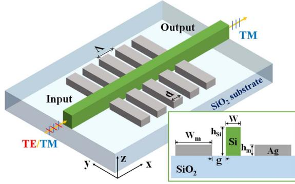
Fig. 1. 3D schematics of proposed TM-pass polarizer. The device is fabricated on SOI platform. Inset: the cross section of the HPG region.
