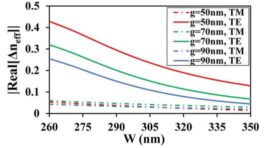
Fig. 2. The absolute value of real part  $\Delta n_{eff}$  for DW and HPW with TM and TE polarization as a function of waveguide width  $W$ . Here,  $h_m = 170$  nm,  $g = 50$  nm, 70 nm and 90 nm, respectively.
