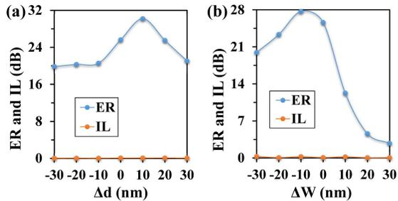
Fig. 6. Dependence of the ER and IL on (a) metal length variation  $\Delta d$  and (b) waveguide width deviation  $\Delta W$
