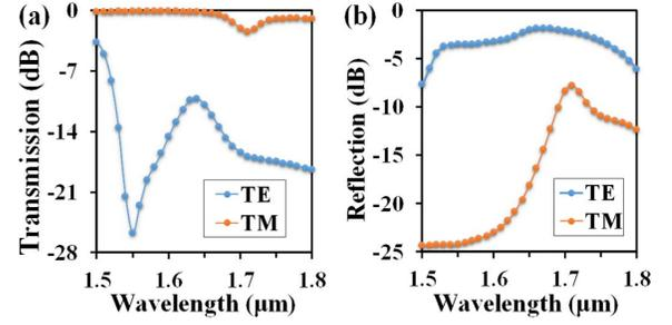
Fig. 5. Wavelength dependence of the transmission (a) and reflection (b) for the proposed TM-pass polarizer.
