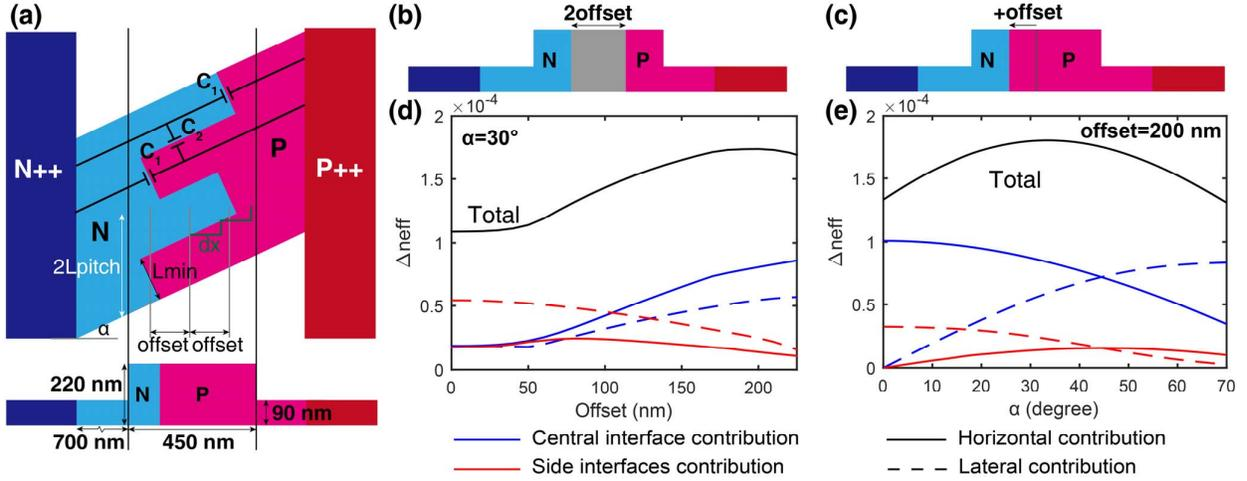
Fig. 1. (a) Schematic of oblique junction, top-view and cross-sectional view. (b) Illustration of 2D simulation of  $\Delta n_h$  and (c)  $\Delta n_l$ . (d) Relations between  $\Delta n_{eff}$  and  $offset$ , at fixed  $\alpha=30^\circ$ . (e) Relations between  $\Delta n_{eff}$  and  $\alpha$ , at fixed  $offset=200$  nm. Doping parameters are  $5 \times 10^{17}/\text{cm}^3$  and  $1 \times 10^{18}/\text{cm}^3$  for P and N doping,  $10^{20}/\text{cm}^3$  for heavy doping.
