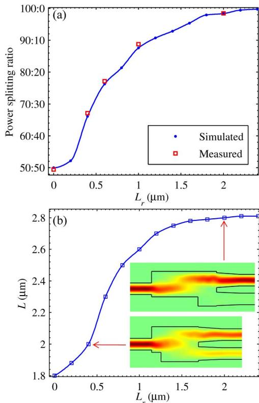
Fig. 3. Relations: (a) PSR at 1550 nm wavelength and (b) corresponding multimode region length ( $L$ ) versus removed rectangle length ( $L_r$ ); the inset shows the optical energy flux density ( $P_z$ ) of an asymmetric MMI splitter with  $L_r = 0.4 \mu\text{m}$  and  $L_r = 2 \mu\text{m}$ .
