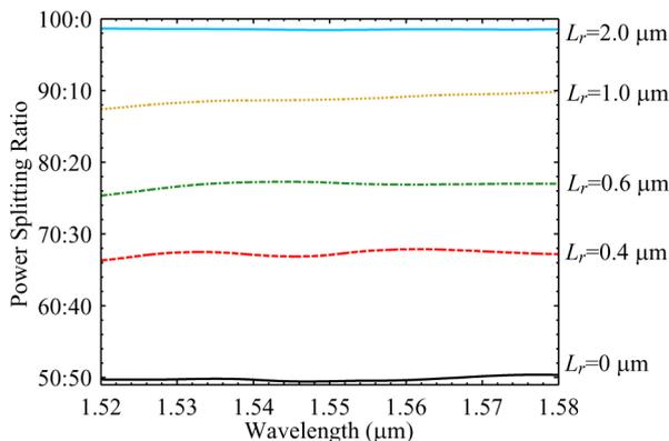
Fig. 4. Wavelength dependence of PSR (measured mean value) at different removed rectangle lengths.
