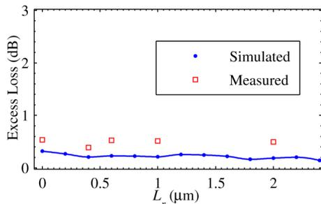
Fig. 5. Excess loss versus removed rectangle length ( $L_r$ ) at 1550 nm wavelength.
