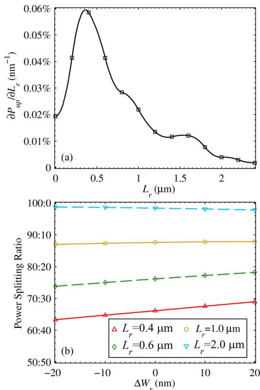
Fig. 6. (a) Derivative of output power from  $\text{WG}_{\text{up}}$  with respect to removed rectangle length ( $L_r$ ) and (b) simulated relations of PSR versus the width variation of removed rectangle ( $\Delta W_r$ ).
